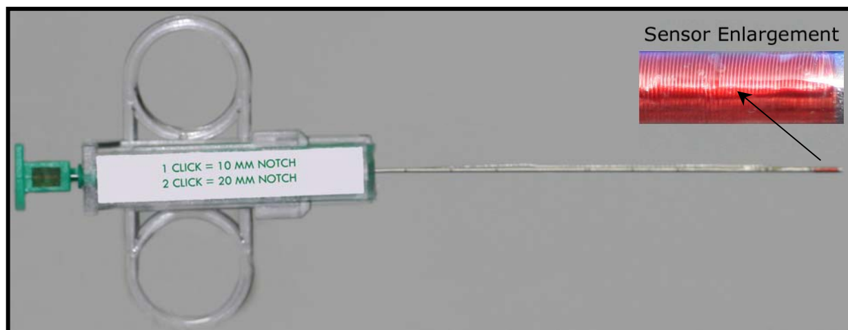
1.15 mm 5DOF sensor integrated onto a 0.9 mm biopsy needle.
